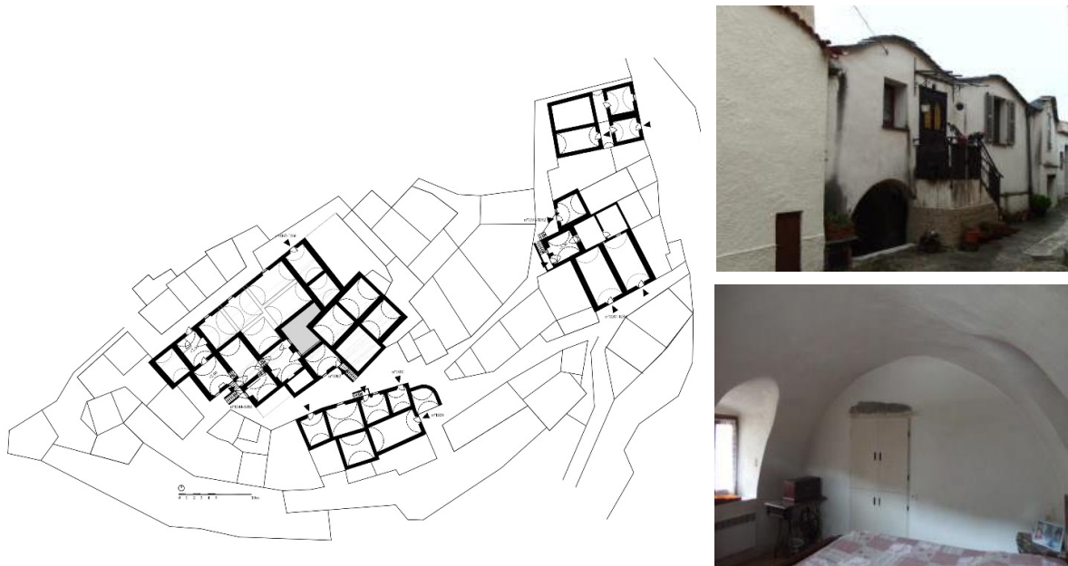
Figure 3: The casun vaulted houses of Breil-sur-Roya region (Maritime Alps, France). Plan of the houses in Cotte village (left). Exterior and interior views of the house with barrel vault with lunettes in street Chemin de Mauriana (right). (Author's drawing and photos)
